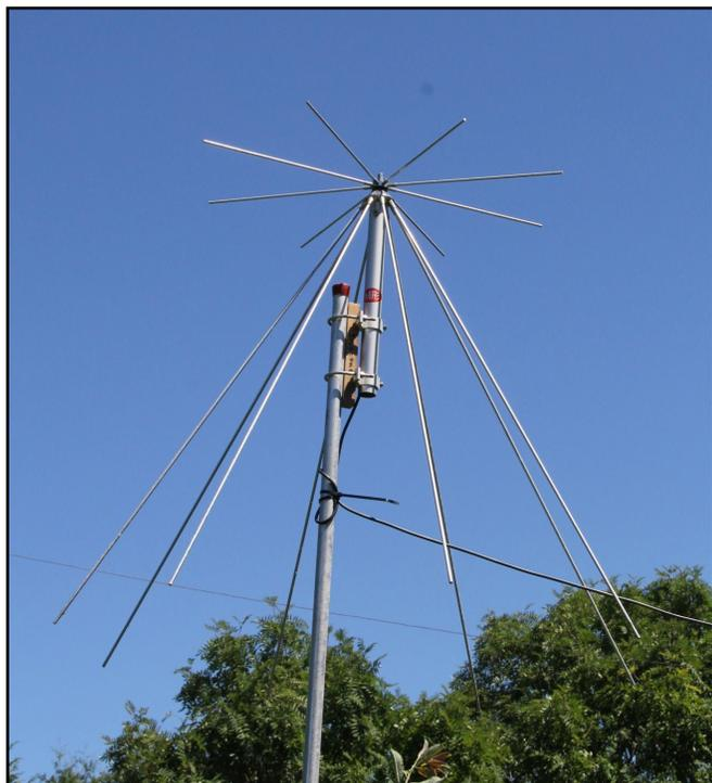
rods inserted into plated fittings that appeared to be made of brass. Once I had gathered the required tools, total assembly time was 15 minutes. The fully assembled antenna is shown above. The antenna is in its second year of use and working well, but the radials show slight weathering due to the salty air in the Gaspé. A spray coat of lacquer would probably provide adequate protection for the time it is exposed to the salt.
